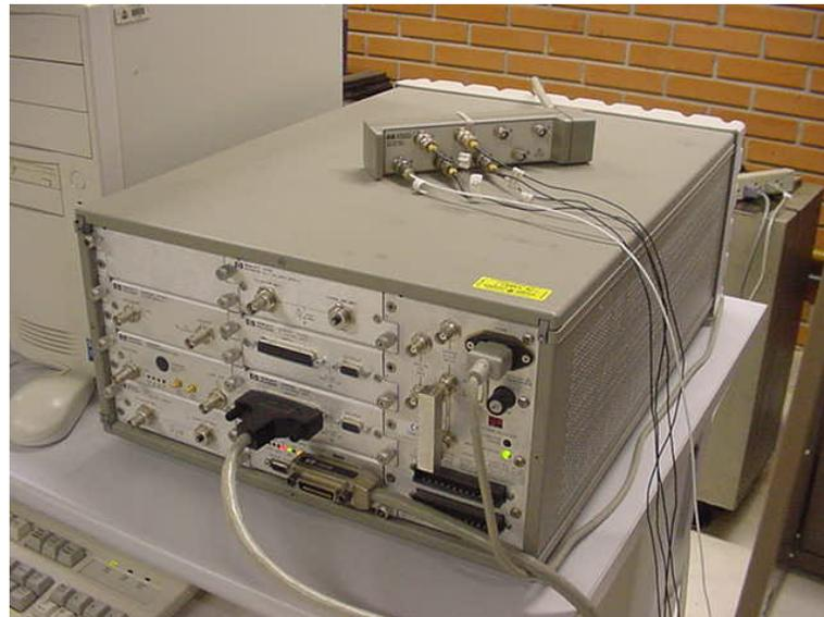
Figura (C.1) - Hewlett Packard (HP) Dynamic Signal Analyzer 3566/67
