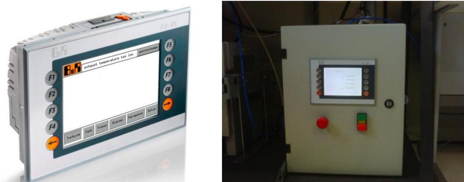
Figura 15 – Conjunto CLP e IHM B&R Automation e Painel de Controle
