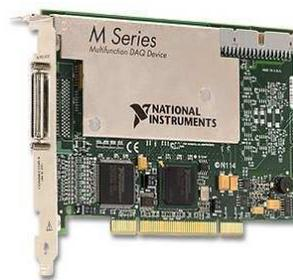
Figura 4.5: Hardware NI PCI-6251.
