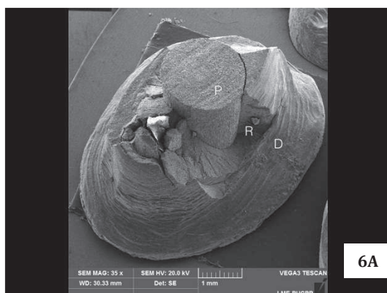
Figure 6-A: Group DZ type III fracture, showing dislocation and fracture of the core filling in the light-polymerized composite resin (R) and post exposure (P) (40×); Figure 6-B: Same specimen showing exposure of the post (P), with no evidence of damage to the remaining tooth structure (D) in the ferrule area (100×).
