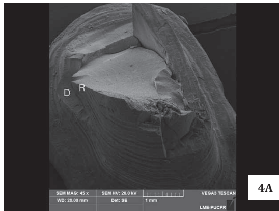
Figure 4-A: Type III fracture in a specimen from the Z group showing more than 50% displacement of the composite resin (R) (40×); Figure 4-B: View of the composite resin fracture, demonstrating no compromise to the integrity of the tooth (D) (100×).
