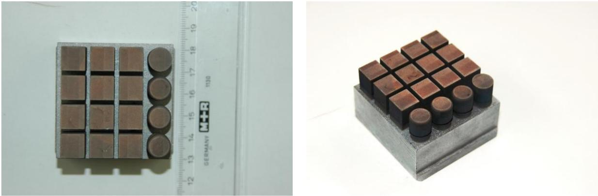
Figure 8.12. SLS parts for EDM experiments.
