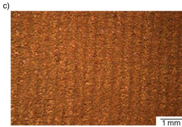
Figure 8.9. Stereomicroscope images of the top of the parts after the hatch distance experiments: a) 0,1 mm, b) 0,2 mm, c) 0,4 mm.
