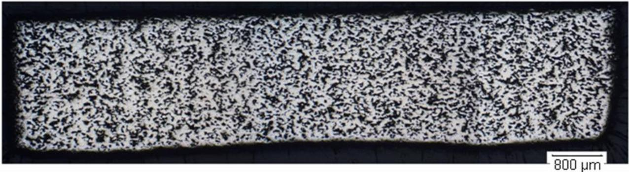
Figure 8.4. Micrographs of the SLS parts after the laser scan speed experiments (the black spaces represent the pores): a) 300 mm/s, b) 250 mm/s, c) 200 mm/s, d) 150 mm/s, e) 100 mm/s, f) 50 mm/s. Magnification 3,2x.
