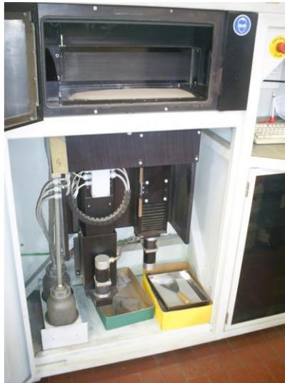
Figure A.5. Sintering machine internal components.
