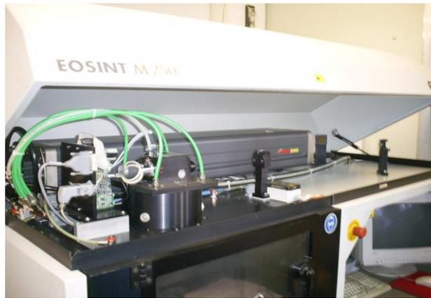
Figure A.7. Sintering machine internal laser components.
