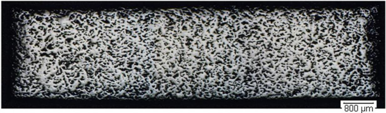
Figure 8.20. Micrograph of the SLS parts: a) Mo 63 wt.% - Cu(100) 37 wt.% mixture, b) Mo 63 wt.% - Cu(90)Ni(10) 37 wt.% mixture, c) Mo 63 wt.% - Cu(70)Ni(30) 37 wt.% mixture. Magnification 3,2x.
