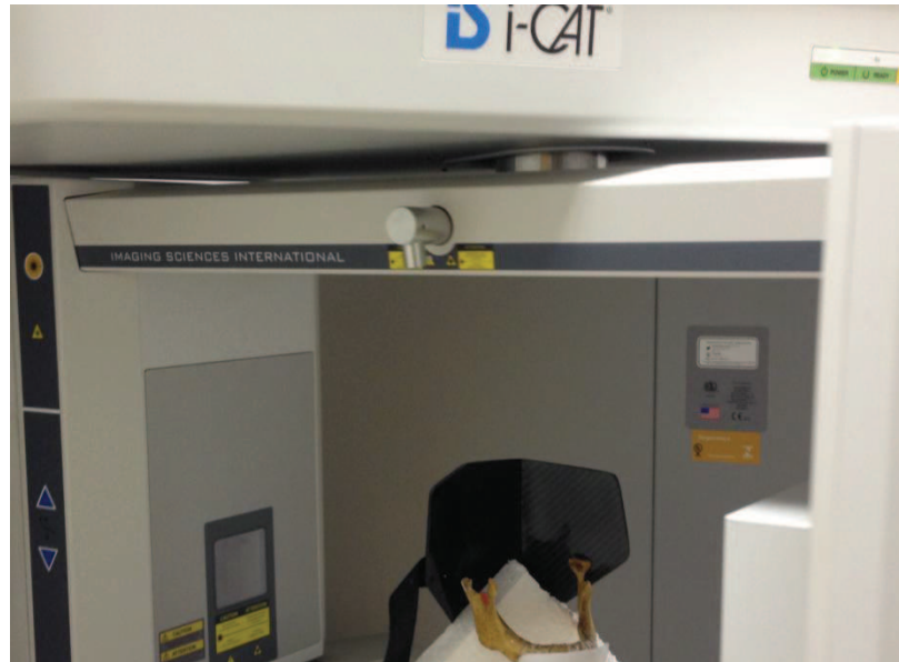
Figure 5 Cone beam tomography scanning (i-CAT 17-19).
