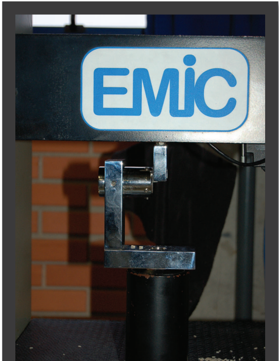
Figure 5: Universal testing machine with the microshear bond strength testing device.
