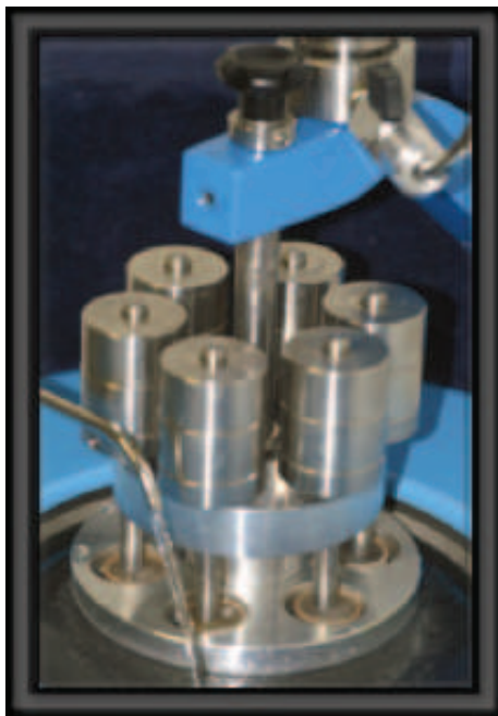
Figure 2: Polishing machine used for the flattening the ceramic specimen surfaces.
