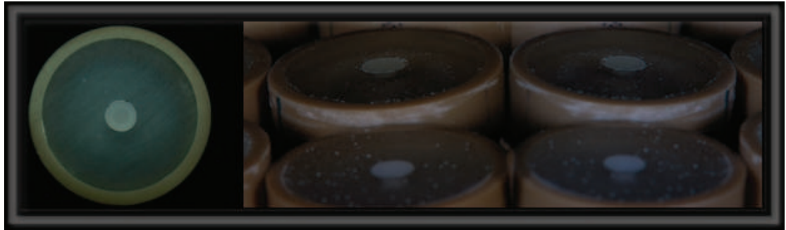
Figure 1: Lithium disilicate ceramic cylinder embedded in acrylic resin.
