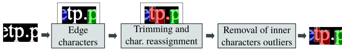
Fig. 2. Overview of the character segmentation procedure. Red boxes delimit inner characters, while blue and green boxes delimit, respectively, the left and right edge characters.
