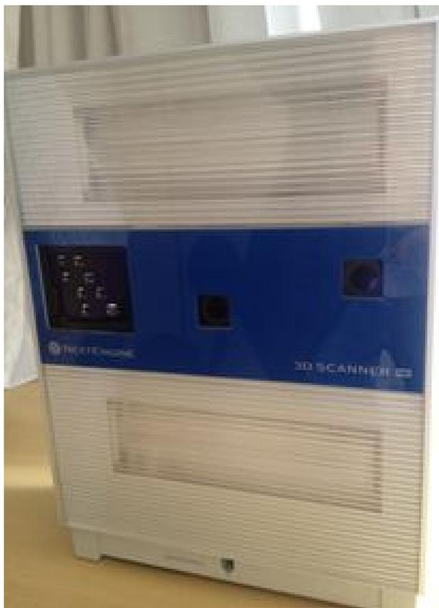
Figura 12: Scanner 3D da NextEngine
