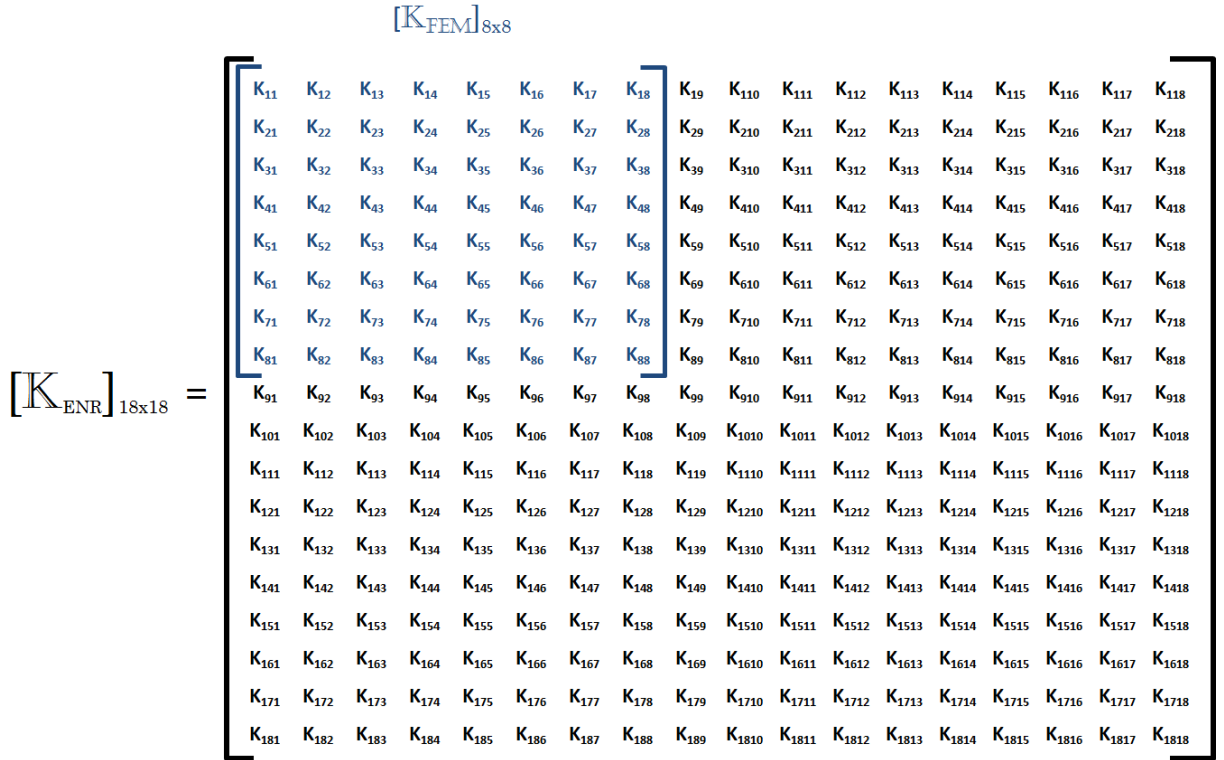
Figure 5.4 – Standard [K_{FEM}] and enriched [K_{ENR}] stiffness matrix.
