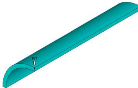
Figure 24 – Model of \frac{1}{4} pipe with pit corrosion
