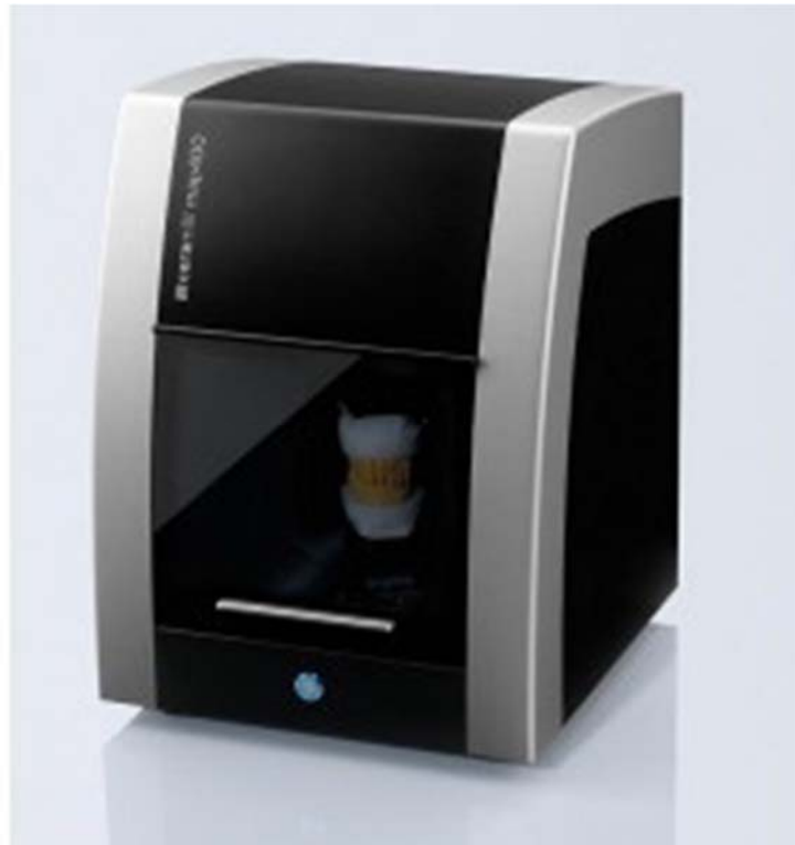
Figure 4: Dental scanner (Ceramill map400, Amann Girrbach, Koblach, Austria)
