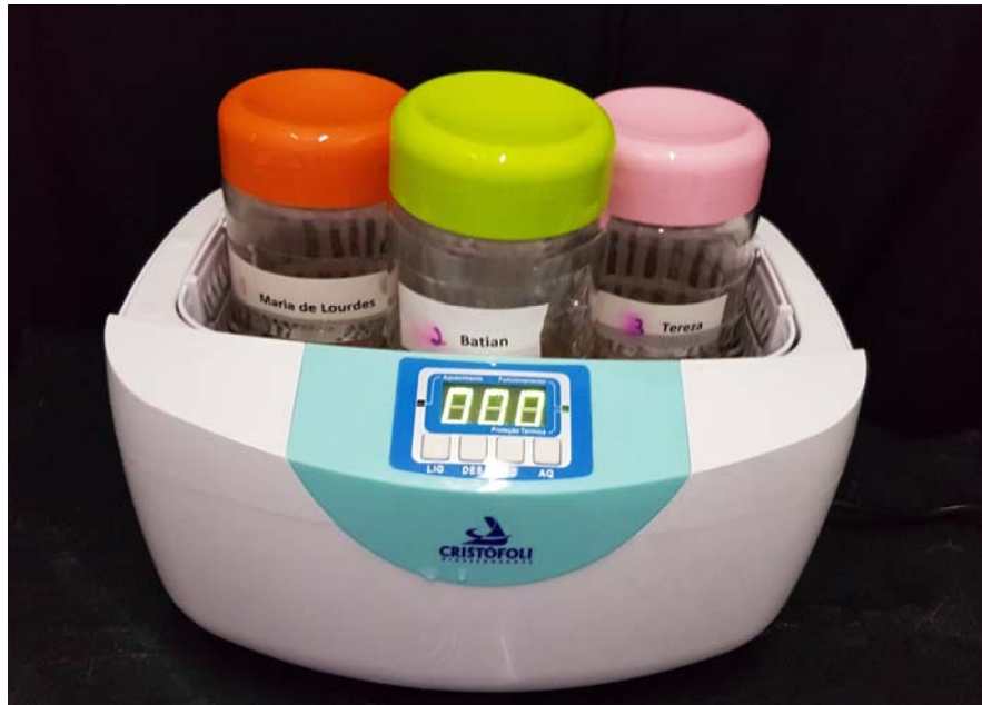
Figure 10: Dentures immersed in physiological saline being sonicated for 15 minutes
