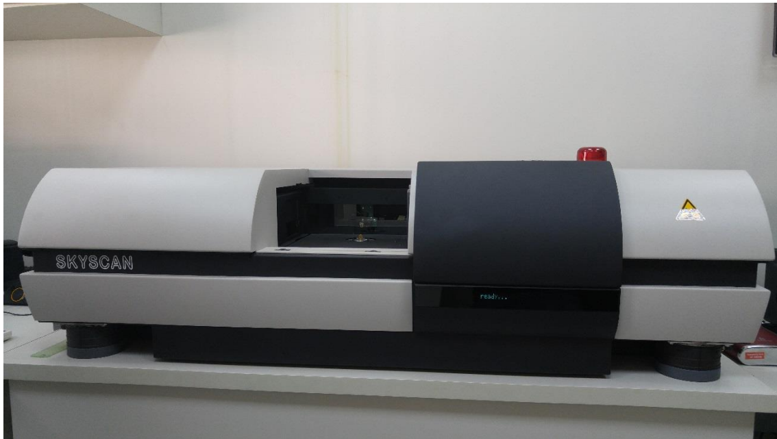
SkyScan 1172, Bruker-microCT, Kontich, Bélgica do LAMIR/UFPR
