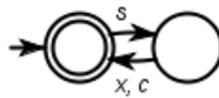
Figura 30 – Task model proposed by (SANTOS et al., 2014): event start ( s ) is controllable, and events complete ( c ) and cancel ( x ) are uncontrollable
