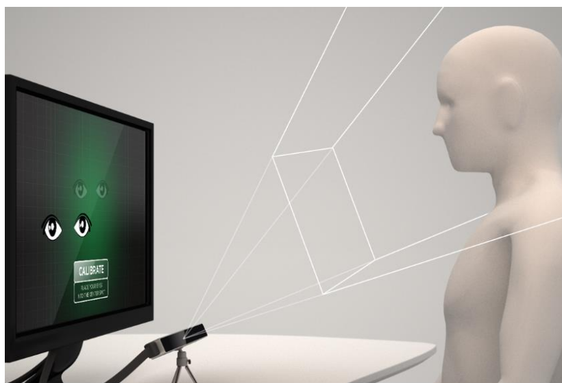
Fig 2. Reach of the sensor guaranteed by the manufacturer and its correct positioning on the lower edge of the monitor
