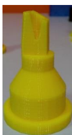
Fig. 1 Glue application nozzle
