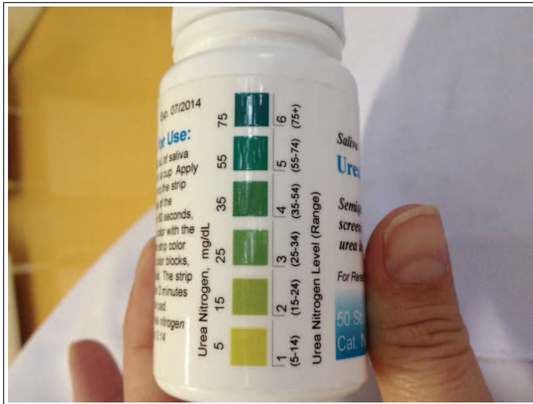
Figure S1: Saliva Urea Nitrogen (SUN) Dipstick reference pads (#1-6) of increasing urea nitrogen range. The change in colour of the test pad is compared to these reference pads.
