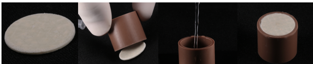
Figure 1. Disc obtained from the glass fiber block embedded on PVC tubes using acrylic resin.
